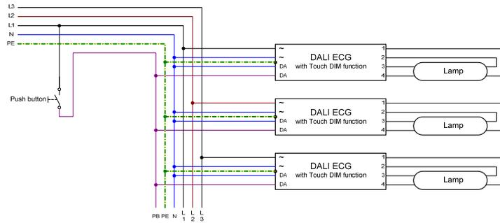
**Fig.:** Up to 4 ECGs can be controlled via Push Button Usage. The number of Push Buttons is limited by the sum of the overall cable length between switch(es) and the connected ECGs which may not exceed 25m.
